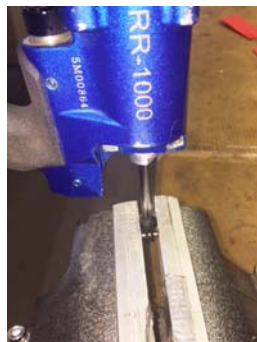
Remove the (4) jaw rollers from the shaft. Do not remove the roller pins. Clamp the shaft (using the roller pins) into a vise.
