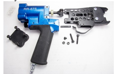
Using a small screwdriver, retract the piston shaft towards the tool body.
