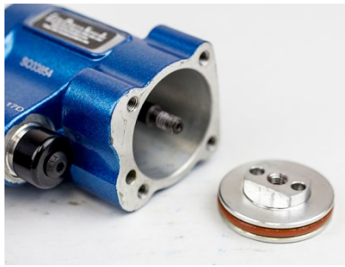
Remove the shaft end plate
