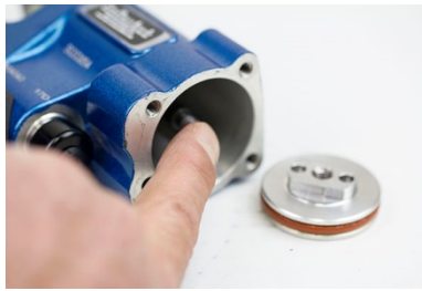
Note: when reinstalling the end plate, apply a “medium” strength thread locker (Loctite) before reinstalling the end plate. Also, apply a little grease on the end plate O-ring before reinstalling.
