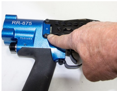
Remove the (4) screws that secure the jaw housing assembly to the tool body
