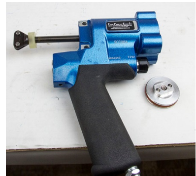
Push the shaft completely out of the tool body.
