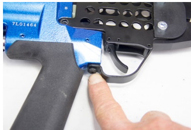
Remove the trigger guard screw
