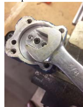
Push the shaft into the tool body so a wrench can access the shaft end plate. This end plate has been installed using Loctite, so it will take some effort to break it loose.
